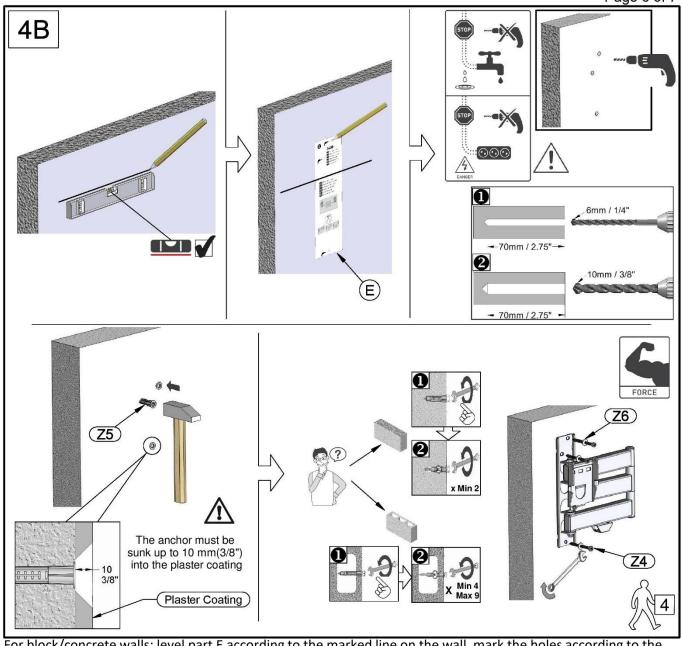
For block/concrete walls: level part E according to the marked line on the wall, mark the holes according to the holes in part E and drill. Connect the part A to the wall.
