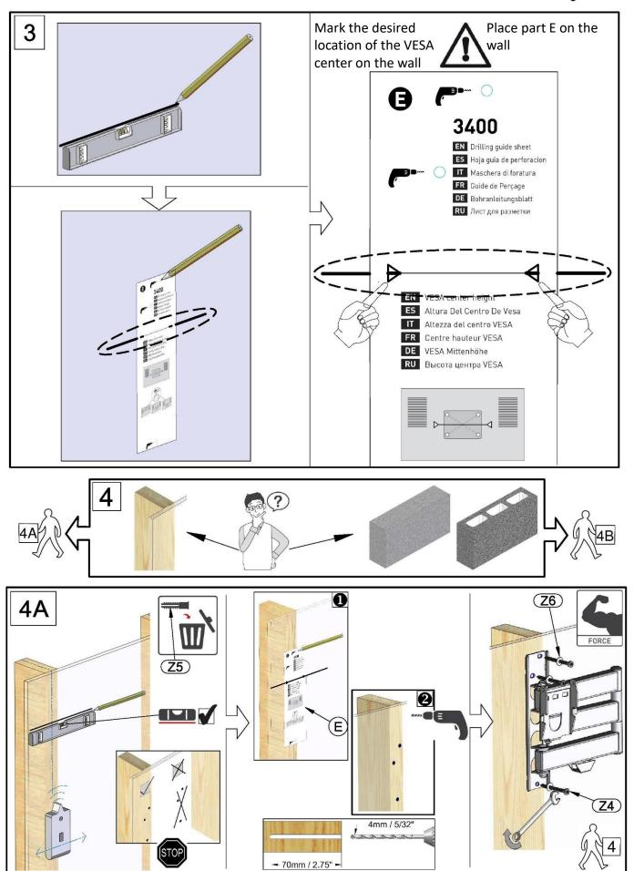
For wood stud walls: Find a stud in the wall, level part E according to the marked line on the wall, mark the holes according to the holes in part E and drill. make sure the wall plate is connected to a stud.
